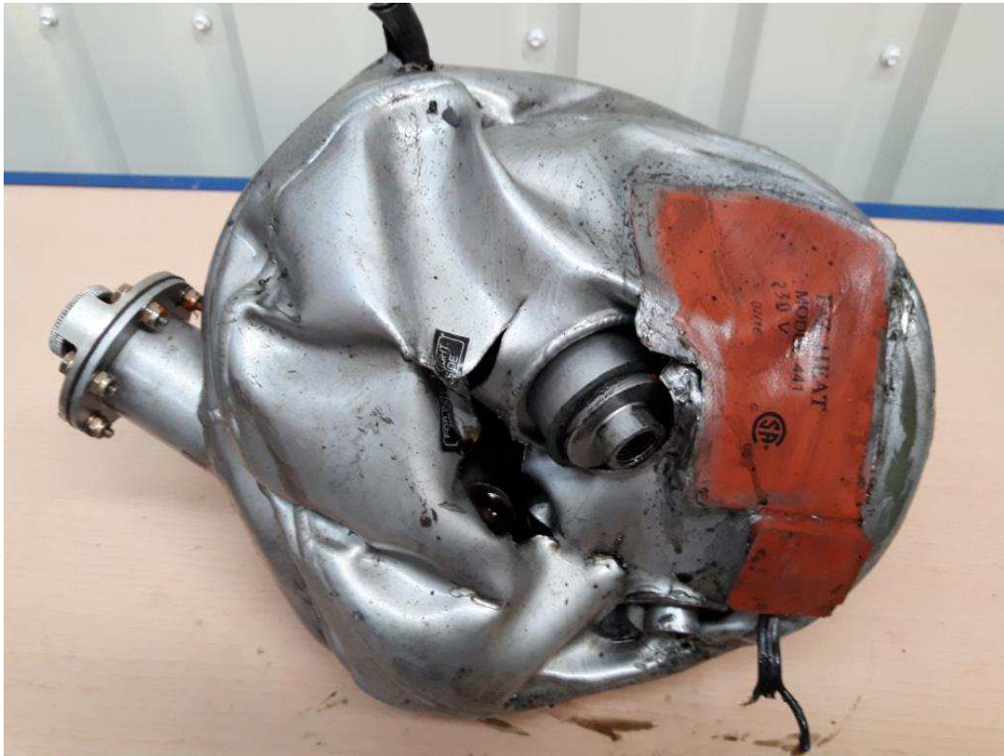
Picture 13 Damaged oil tank
