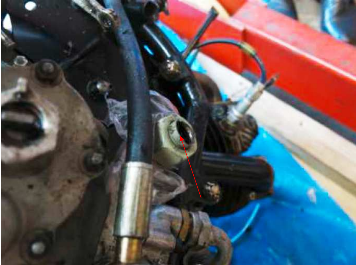
Broken fitting on the oil pump (to oil filter)
