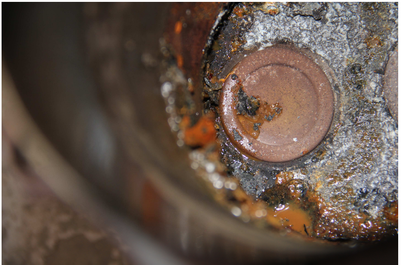
Piston #6 with severe plague and corrosion
