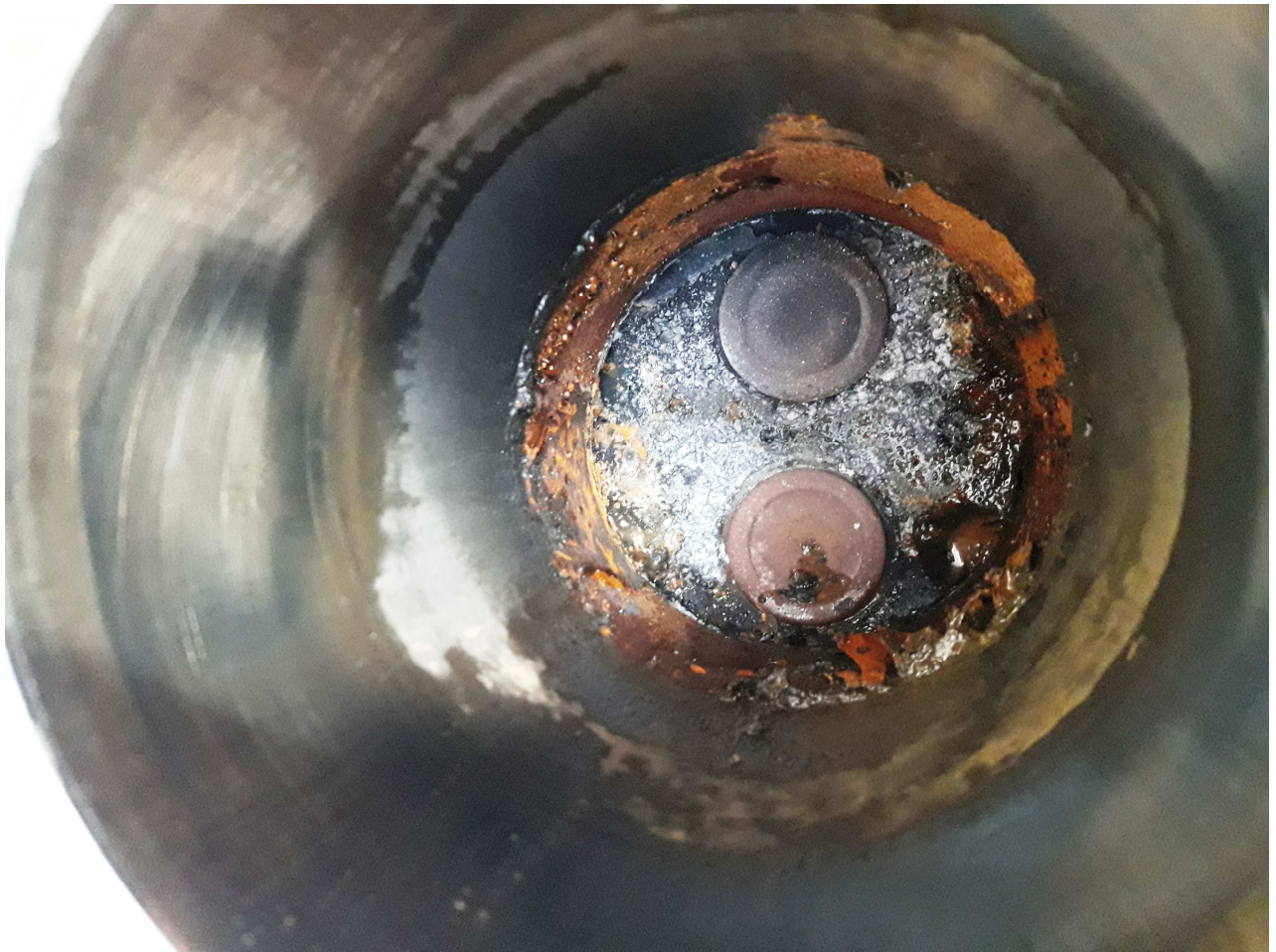
Piston #6 with severe plague and corrosion
