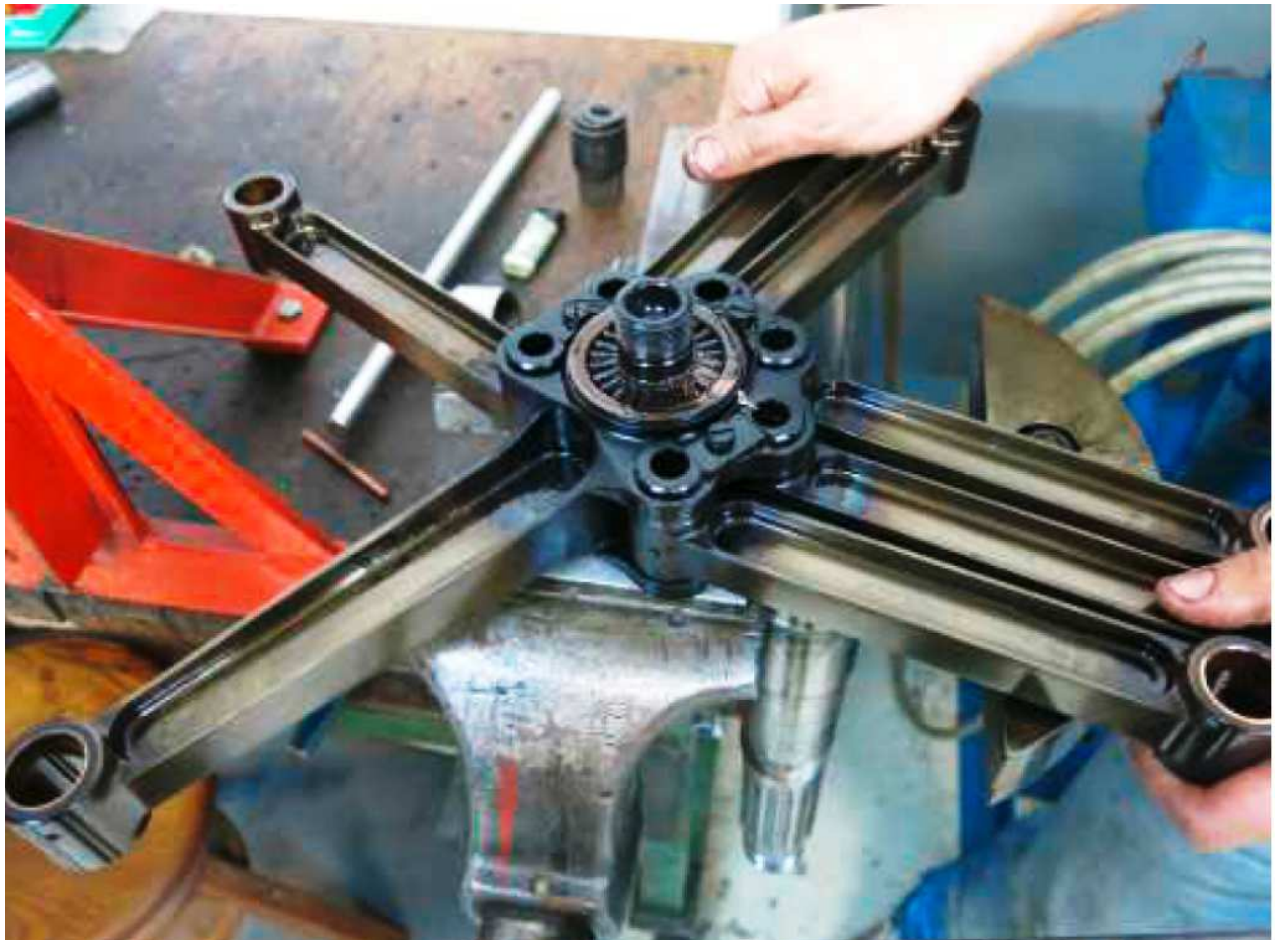
Piston rod assembly- blue colour marks on lower and upper end
