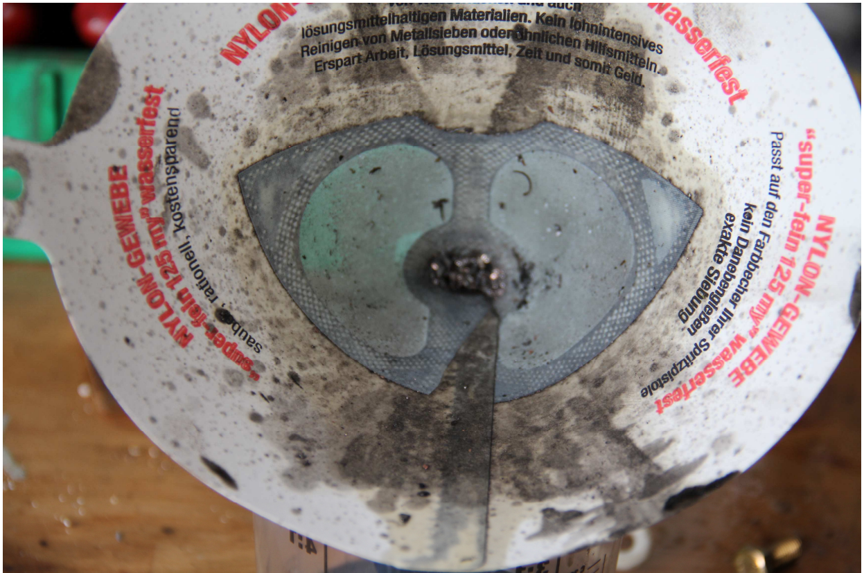
Coarse filter was loose and not secured. There was a noticeable amount of water in filter housing. There were found metallic particles in the filter – mostly bronze colour.
