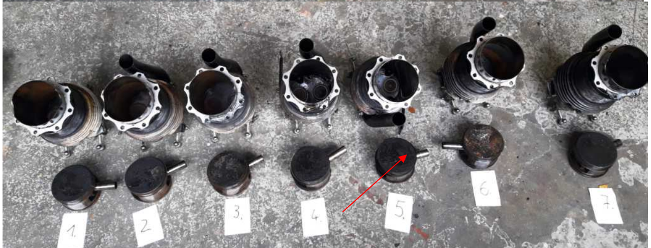
Cylinder 6 with signs of corrosion
