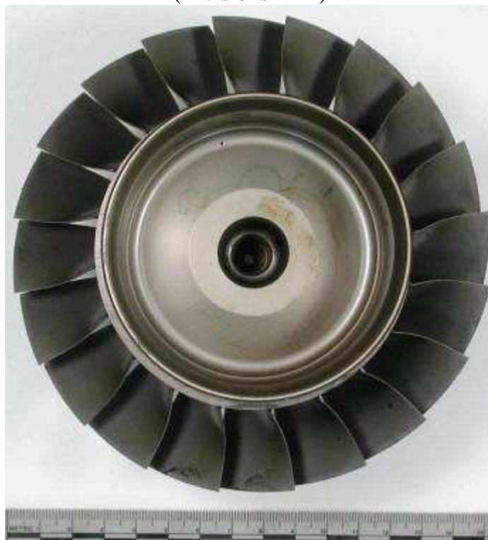
Figure 67 The image of the shows the trailing edge surface of the stage 1 compressor wheel (Divisions=mm)
