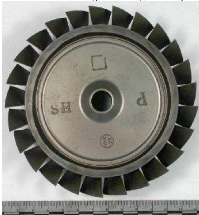
Figure 77. The image of the leading edge surface of the stage 4 compressor wheel. Divisions = mm
