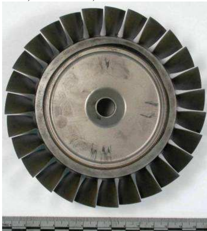
Figure 69. The image of the leading edge surface of the stage 2 compressor wheel (Divisions = mm)
