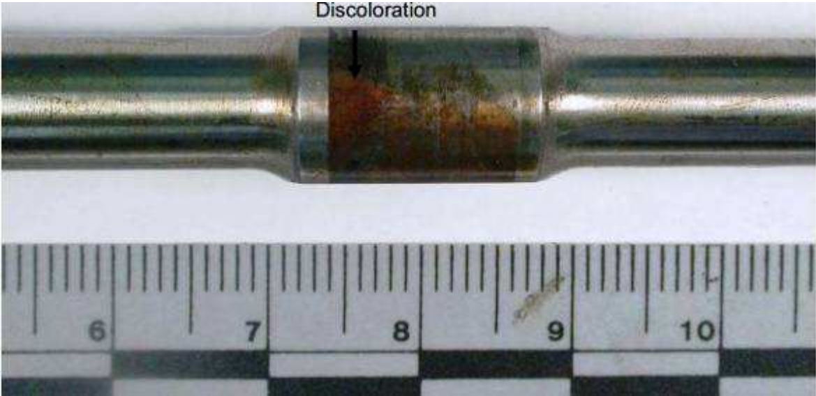
Figure 96. The image of the compressor tie bolt (top) and localized discoloration on the mute area (bottom), Divisions = mm.
