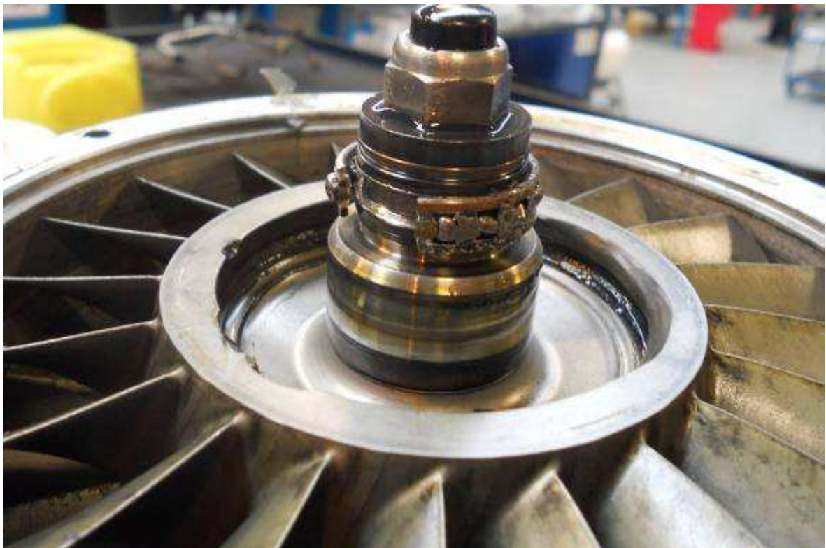
Figure 35. Damaged No1 bearing.
