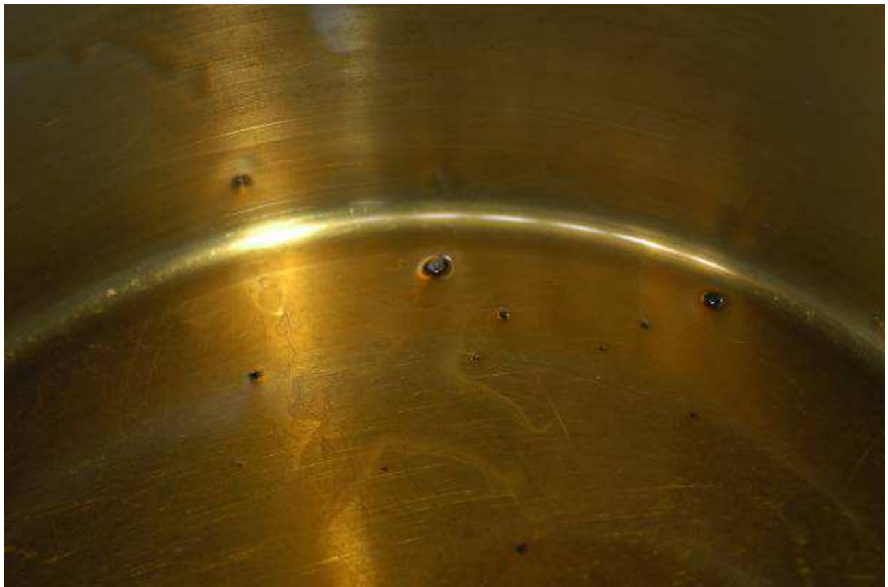
Figure 25. Pieces of metal in the poured oil from engine
