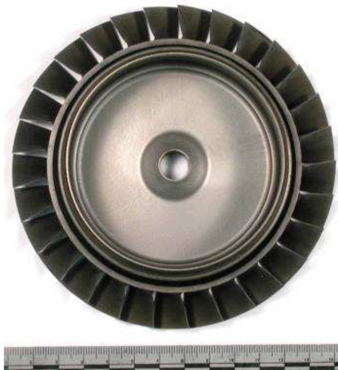
Figure 74. The image of the trailing edge surface of the stage 3 compressor wheel (Divisions = mm)
