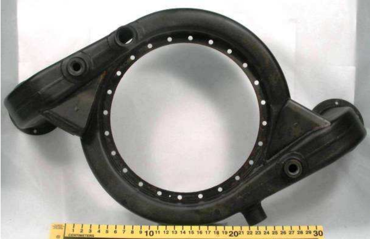
Figure 102. The image of the conditions of the scroll assembly from the forward face. Divisions = cm
