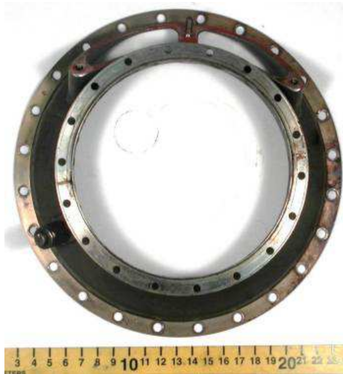
Figure 101. The image of the condition of the bleed manifold as viewed from the forward face. Divisions = cm
