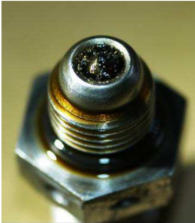
Figure 27. Metallic chips on the upper chip detector
