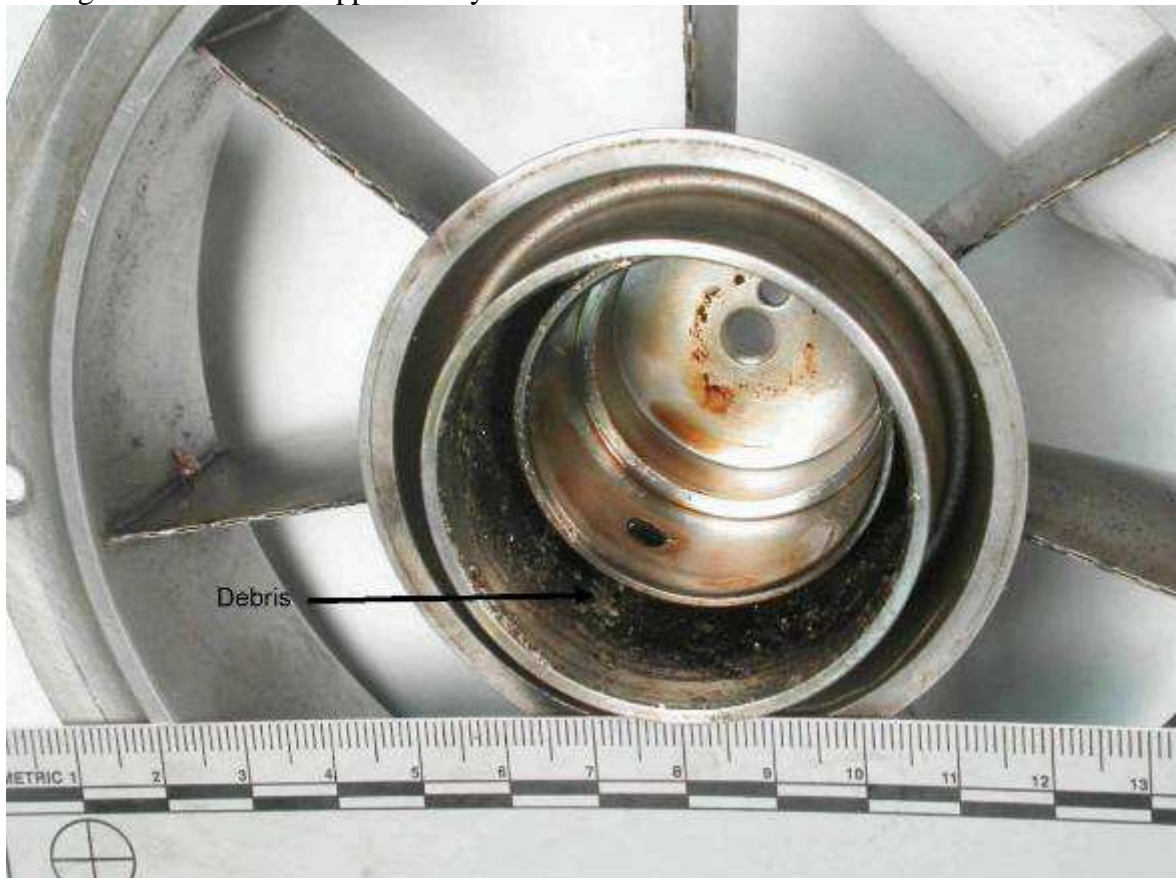
Figure 47. After the bearing housing assembly had been removed.
