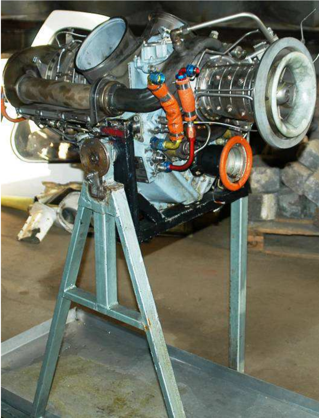
Figure 20 Removed engine on the stand for disassembling into sections
