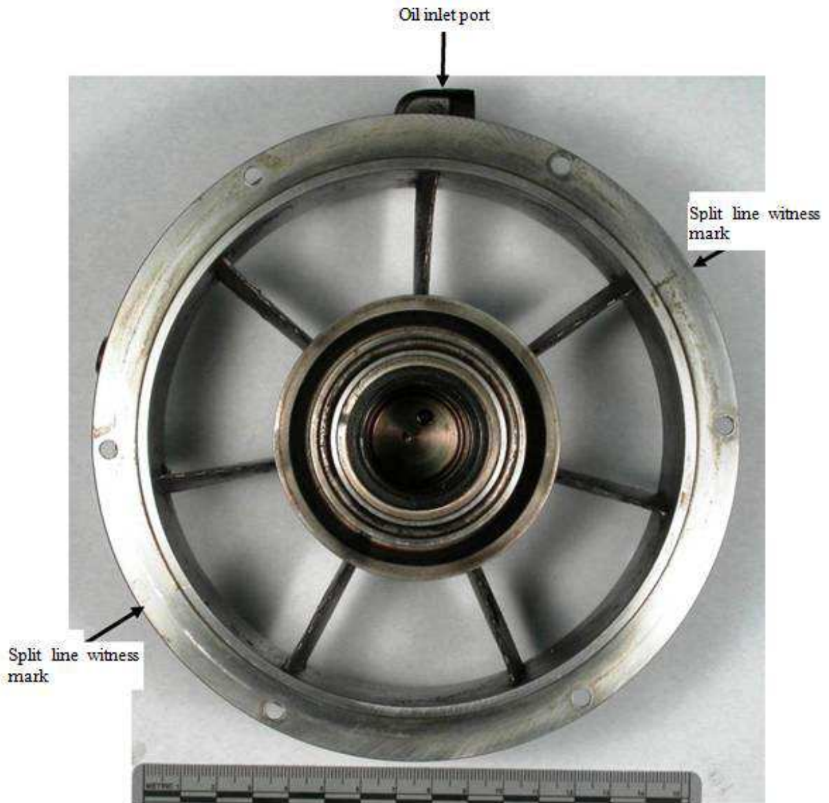
Figure 45. The front compressor support assembly viewed from the aft side
