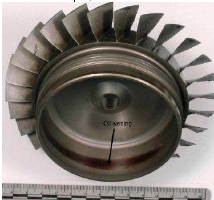
Figure 71. The image of the oil wetting within the aft inner diameter of the stage 2 compressor wheel. Divisions = mm
