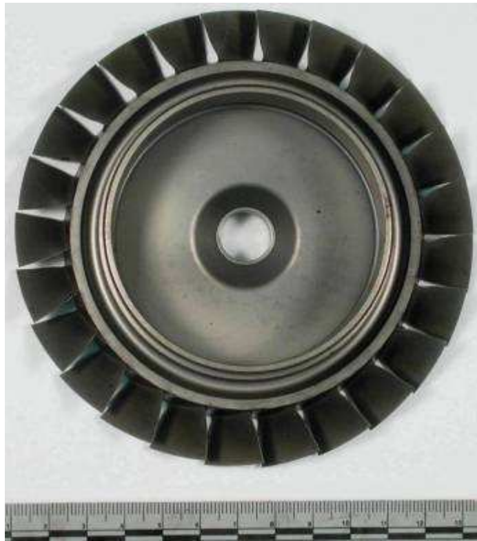
Figure 78. The image of the leading edge surface of the stage 4 compressor wheel. Divisions = mm
