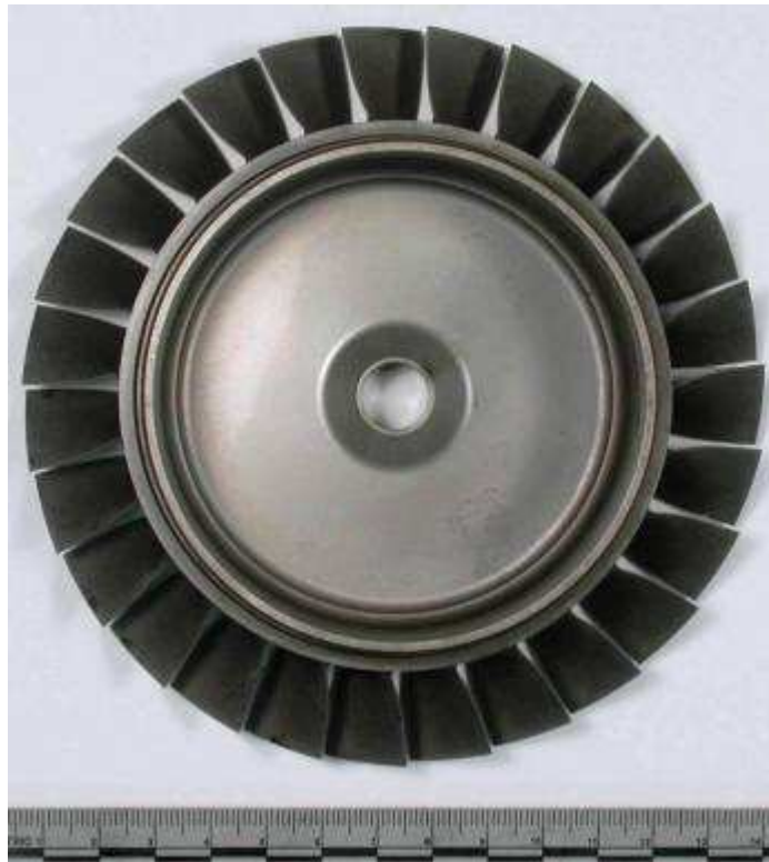
Figure 70. The image of the trailing edge surface of the stage 2 compressor wheel (Divisions = mm)
