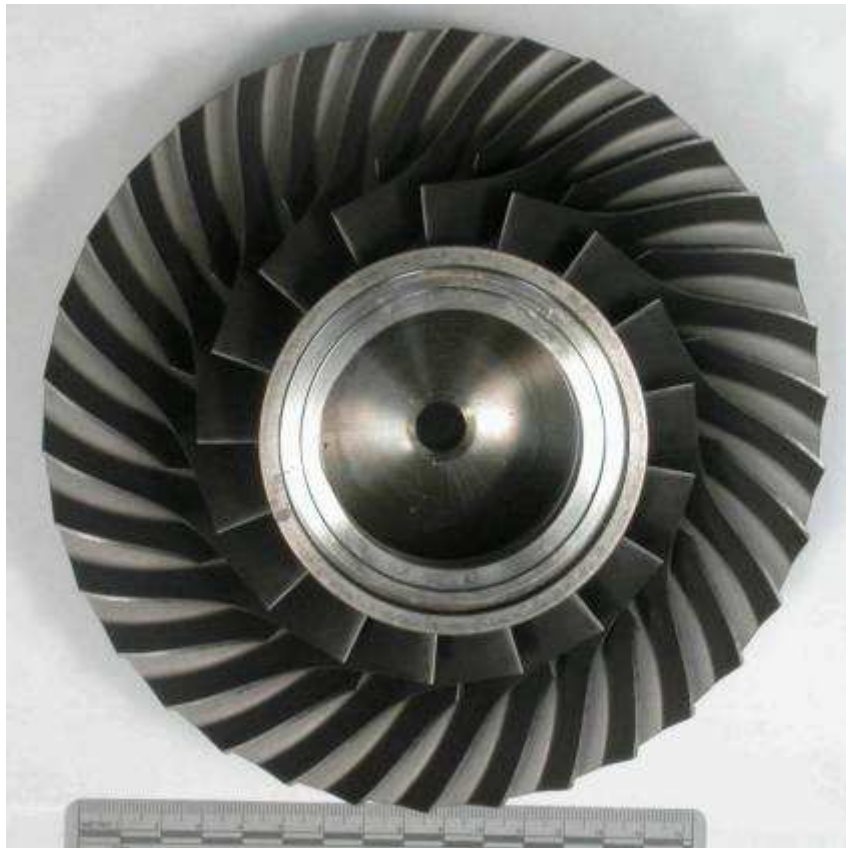
Figure 80. The image of the condition of the impeller as viewed from the forward face. Divisions = mm
