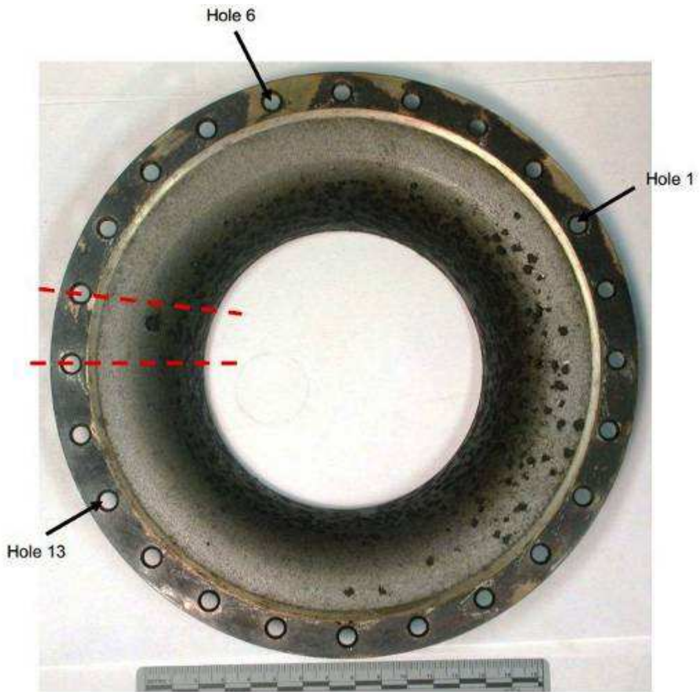
Figure 87. The image of the impeller shroud from the aft face. The red dashed lines represent the plane of metallurgical sectioning. (Divisions = mm)
