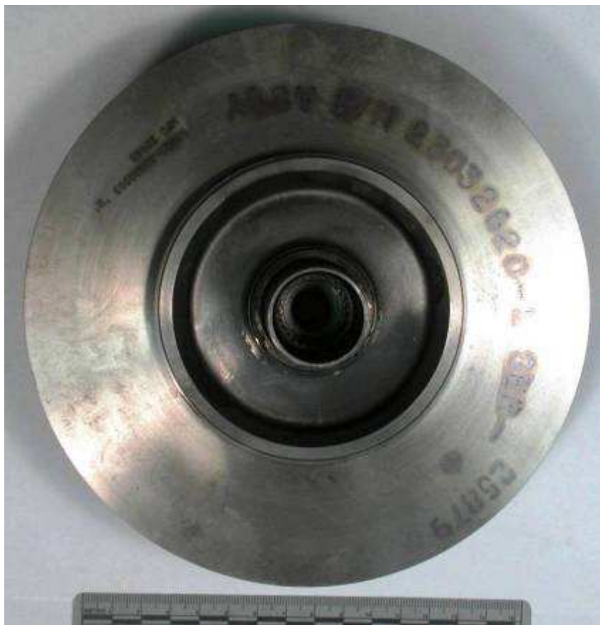
Figure 81. The image of the condition of the impeller as viewed from the aft face. (Divisions = mm)
