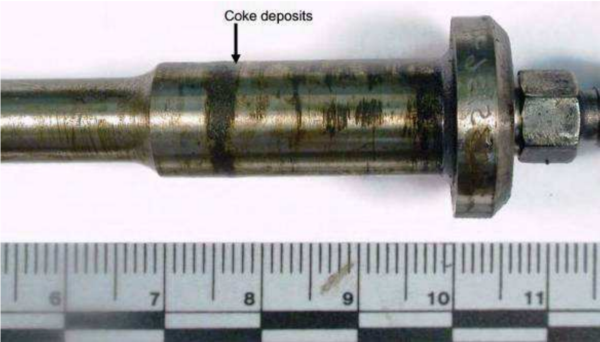
Figure 97. The image of the coke deposits on the end of the compressor tie bolt. (Divisions – mm)
