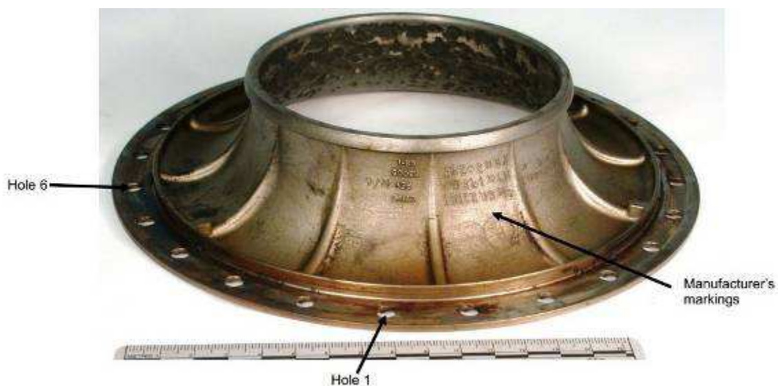
Figure 85. The image of the impeller shroud as viewed from an oblique view to the forward face. Divisions = mm
