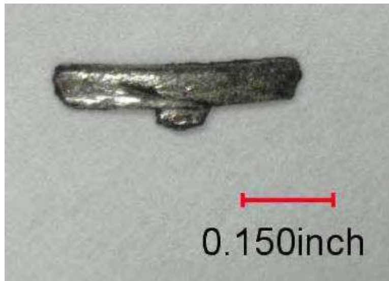
Figure 49. The debris flushed and collected from both the front compressor support and the bearing housing assembly.
