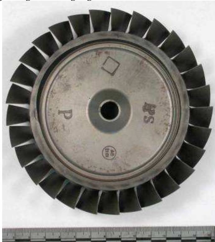
Figure 73. The image of the leading edge surface of the stage 3 compressor wheel (Divisions = mm)
