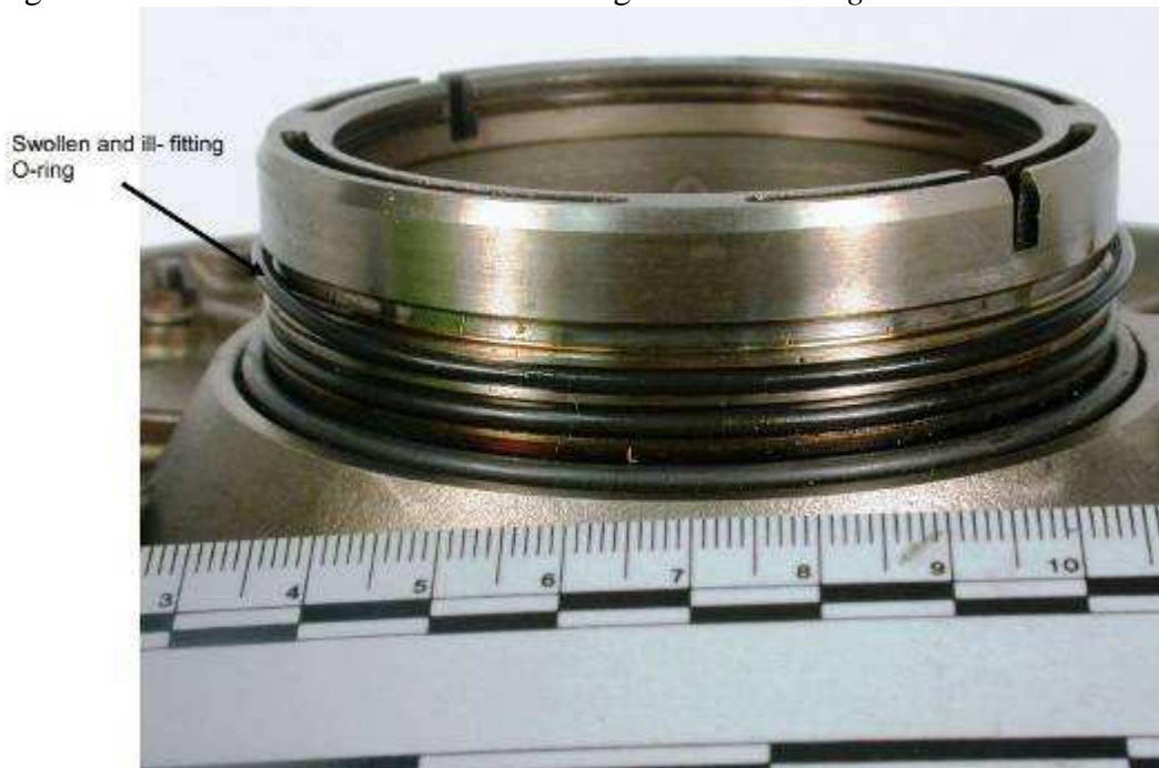
Figure 100 The image of the loose fitting O-ring on the compressor rear support and diffuser as viewed from the aft face
