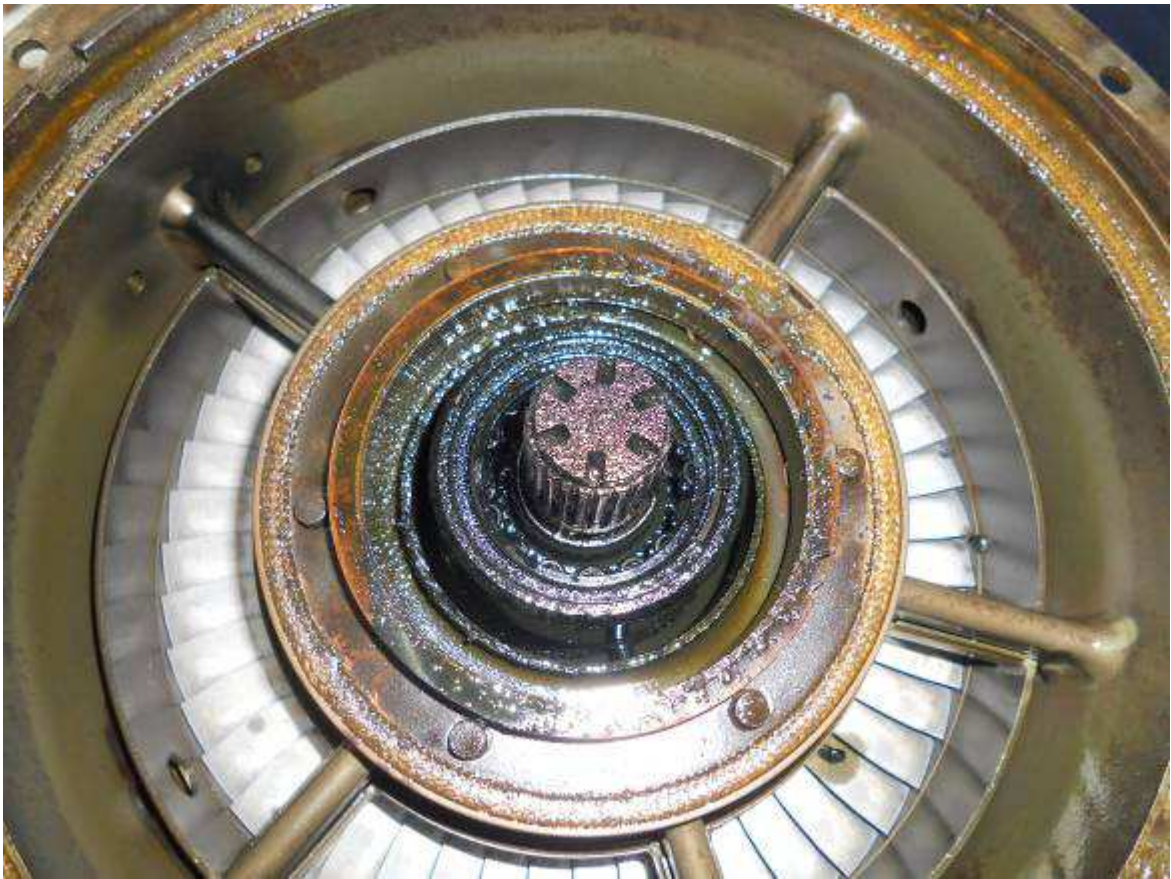
Figure 39. Heavy concentration of diffused material
