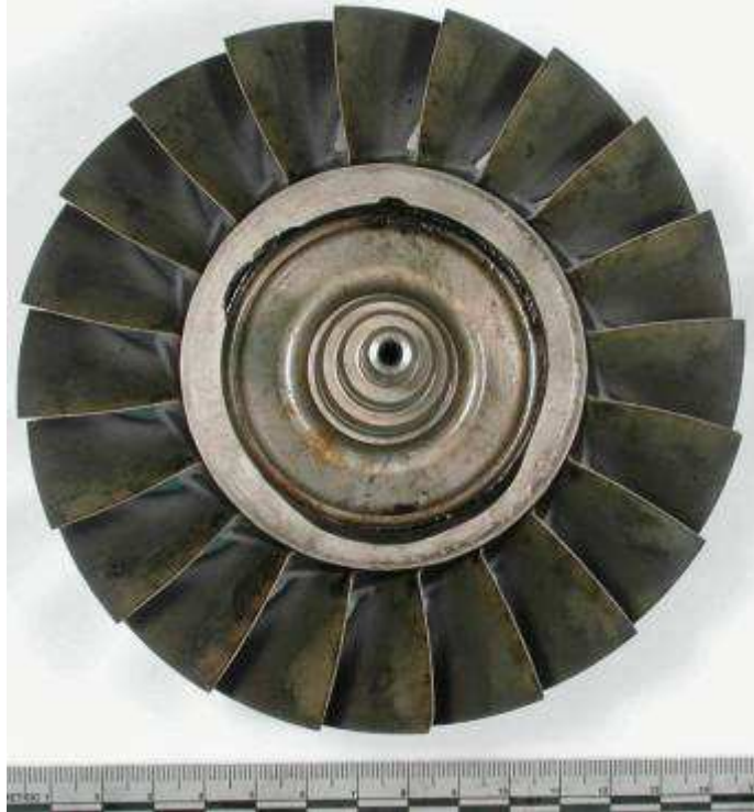
Figure 66 The image of the leading edge surface of the stage 1 compressor wheel (Divisions=mm)
