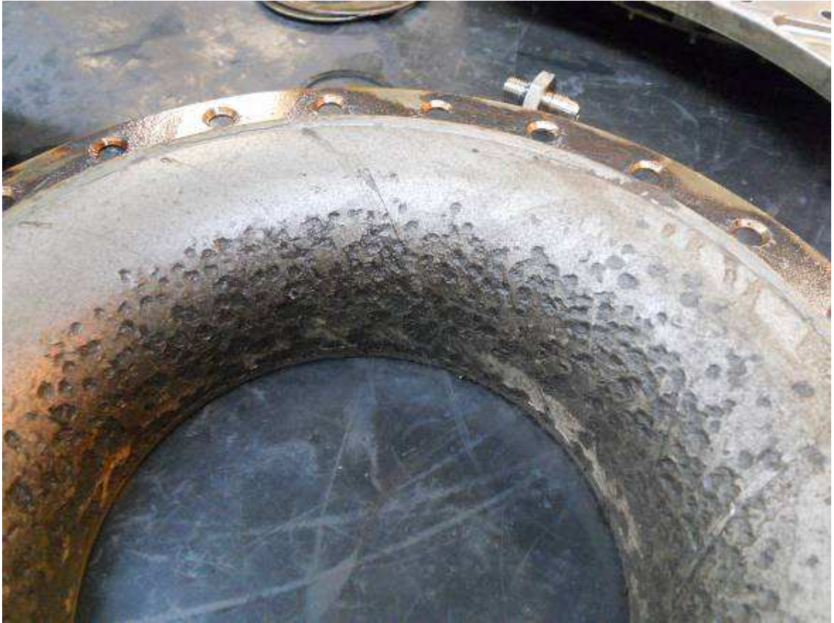
Figure 41 Front shroud damage to coating
