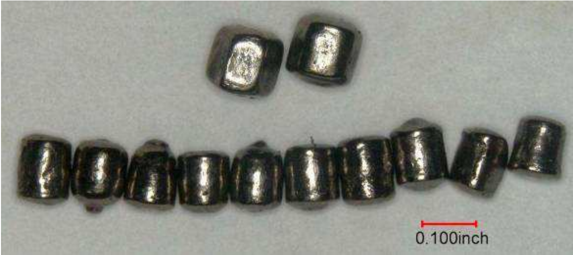
Figure 52 The variety of damage that the 12 (twelve) of rollers exhibited from the No1 bearing. Two rollers had undergone metallurgical evaluation and were unavailable for the photograph.
