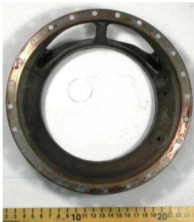
Figure 102. The image of the condition of the bleed manifold as viewed from the aft face. Divisions = cm
