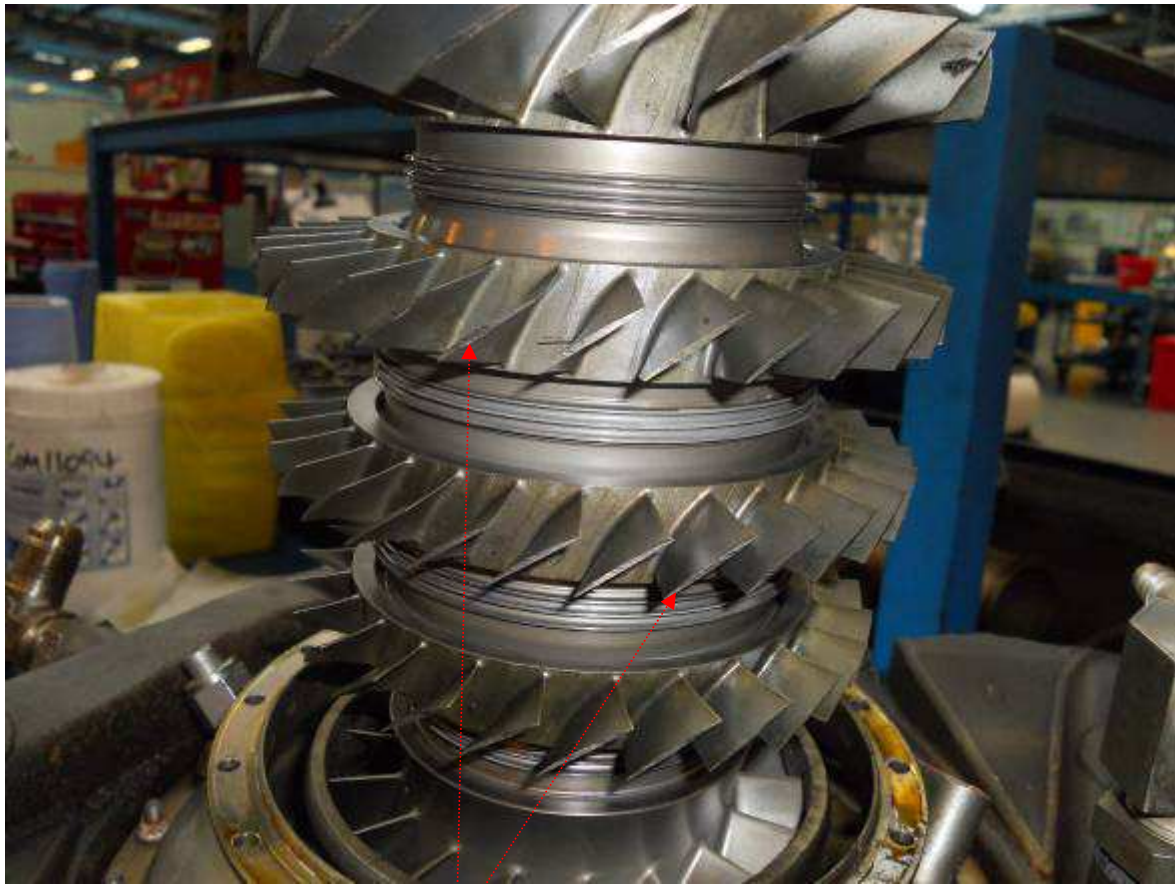
Figure 43. Blades tip rub on the stage 1 compressor wheel contact
