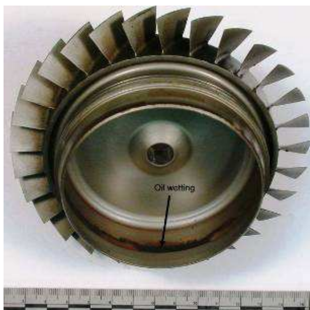
Figure 75. The image of the oil wetting within the aft inner diameter of the stage 3 compressor wheel. (Divisions = mm)
