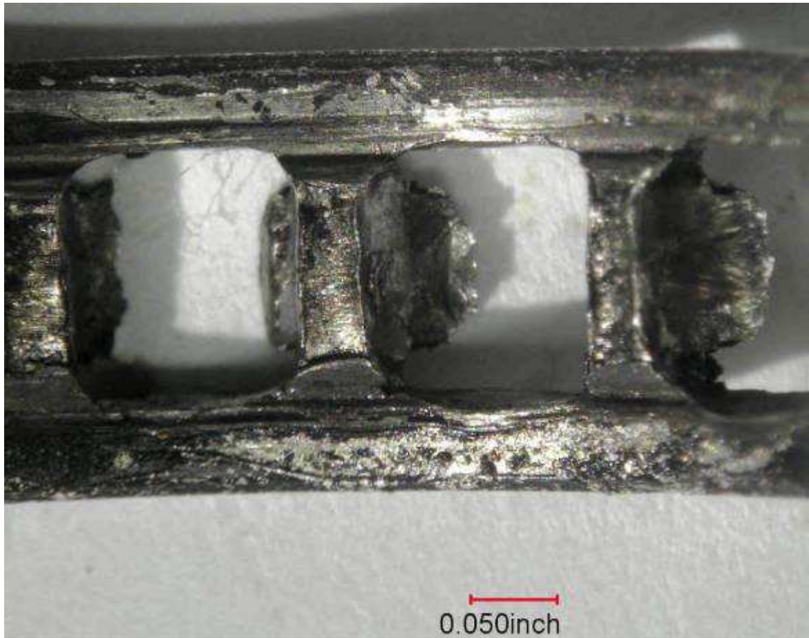
Figure 58. Wear deformation from the inner surface of the No. 1 bearing separator pockets.
