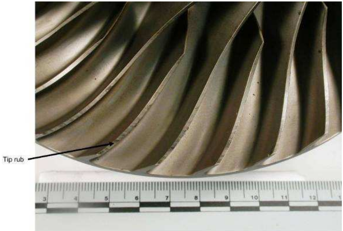
Figure 82. The image of a representative example of tip rub on the impeller. (Divisions = mm)
