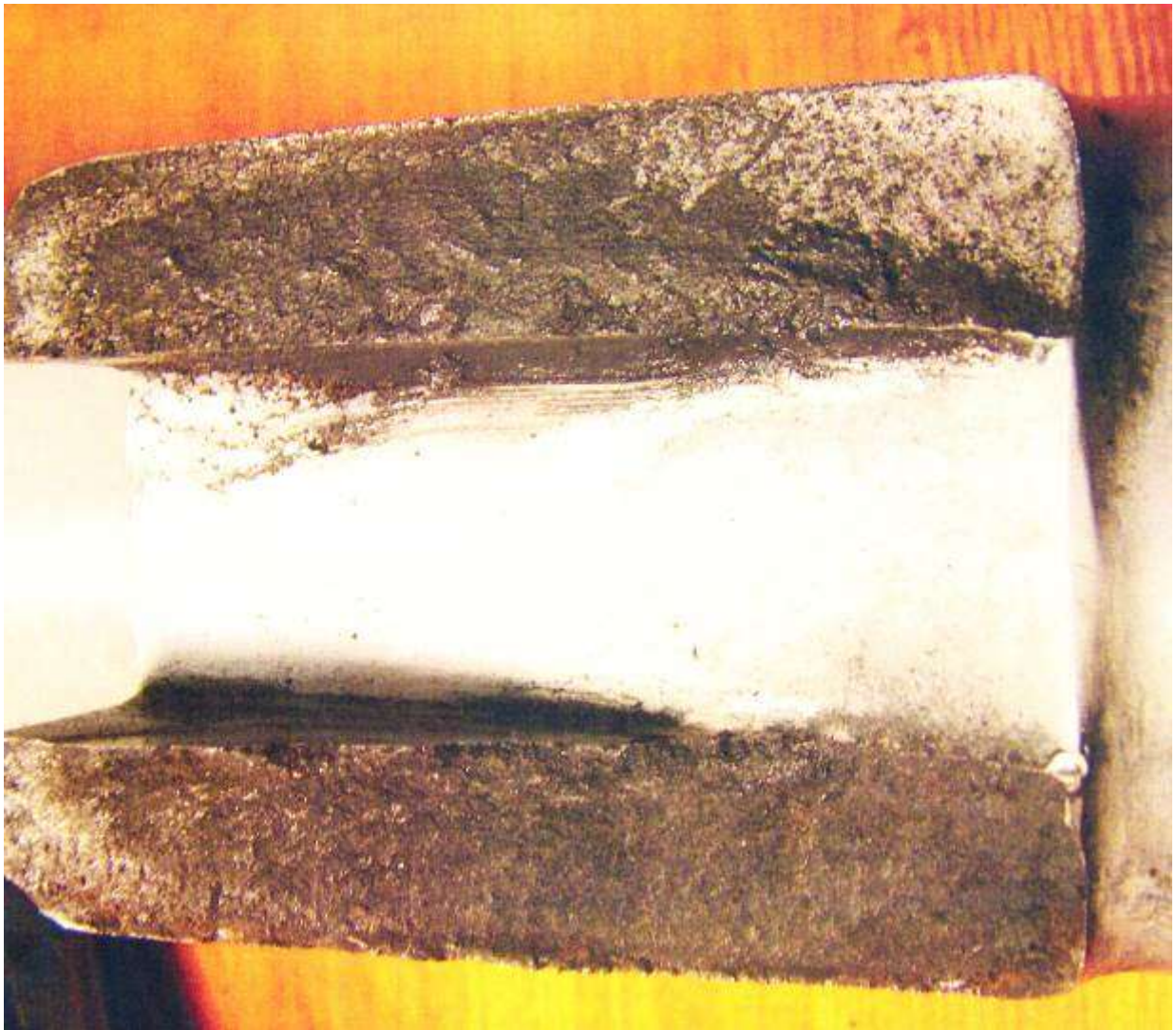
Figure 8. Fracture overview magnified twice
