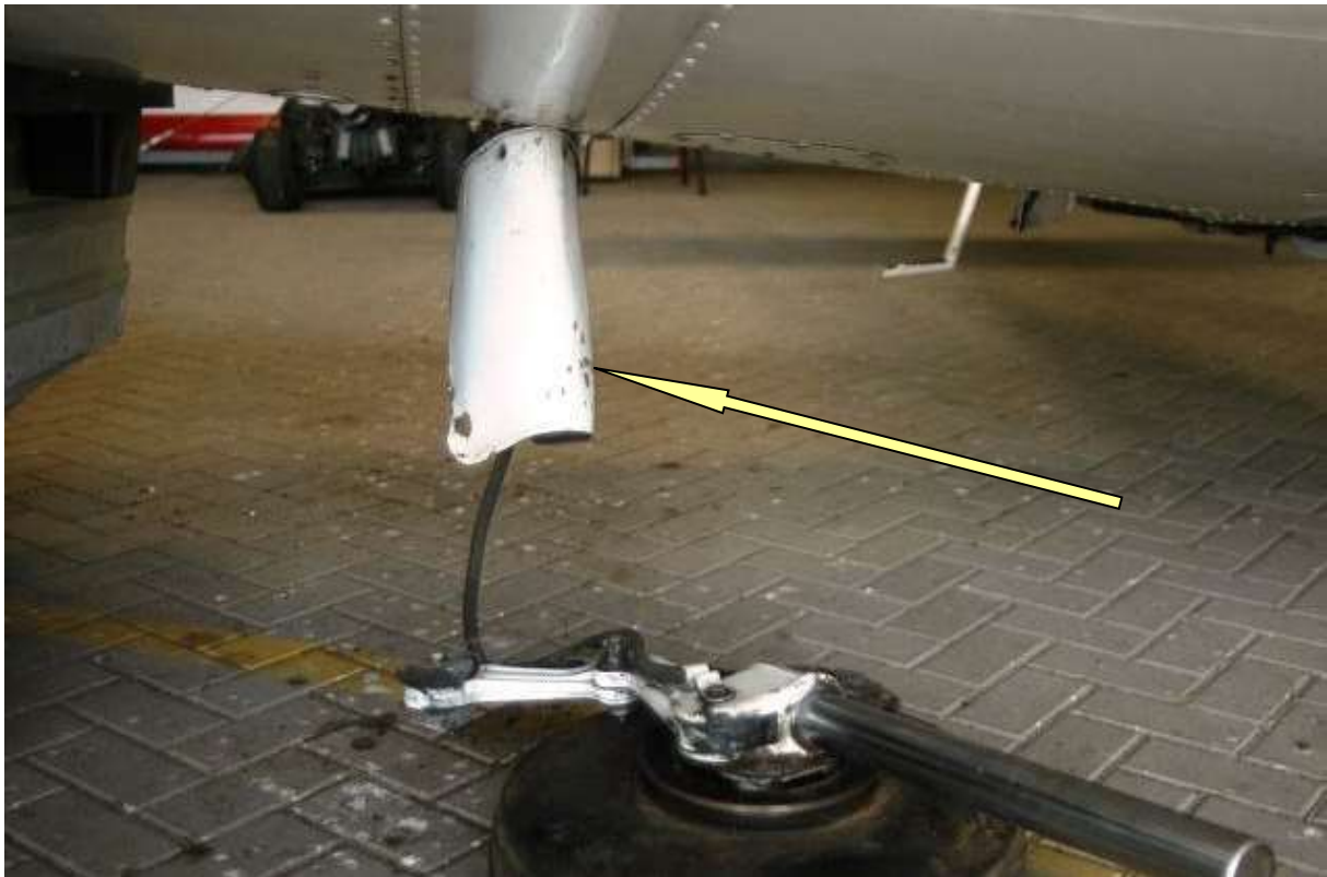
Figure 3. Protective shield of the right-hand landing gear strut cylinder
