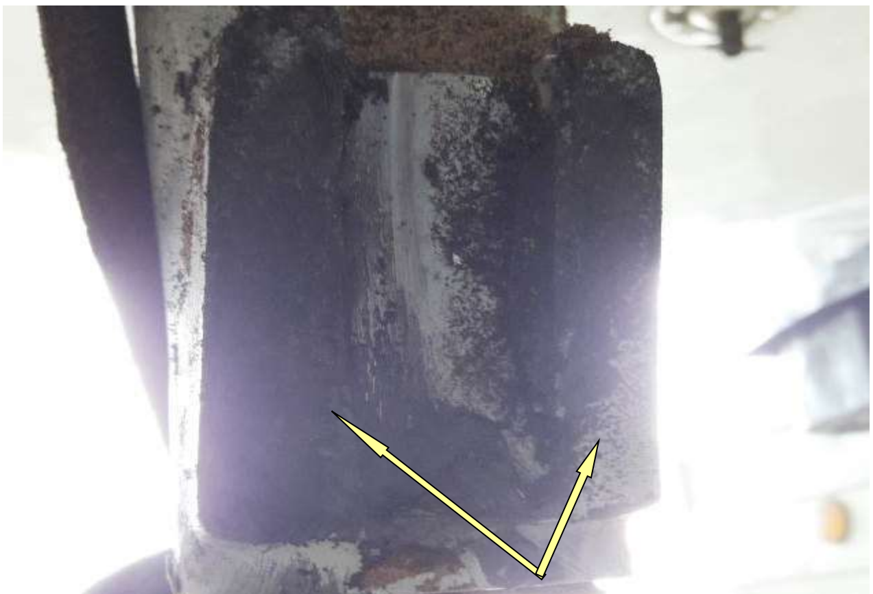
Figure 4. Breaking points of the torque link lugs (ear) at oleo cylinder of right-side landing gear
