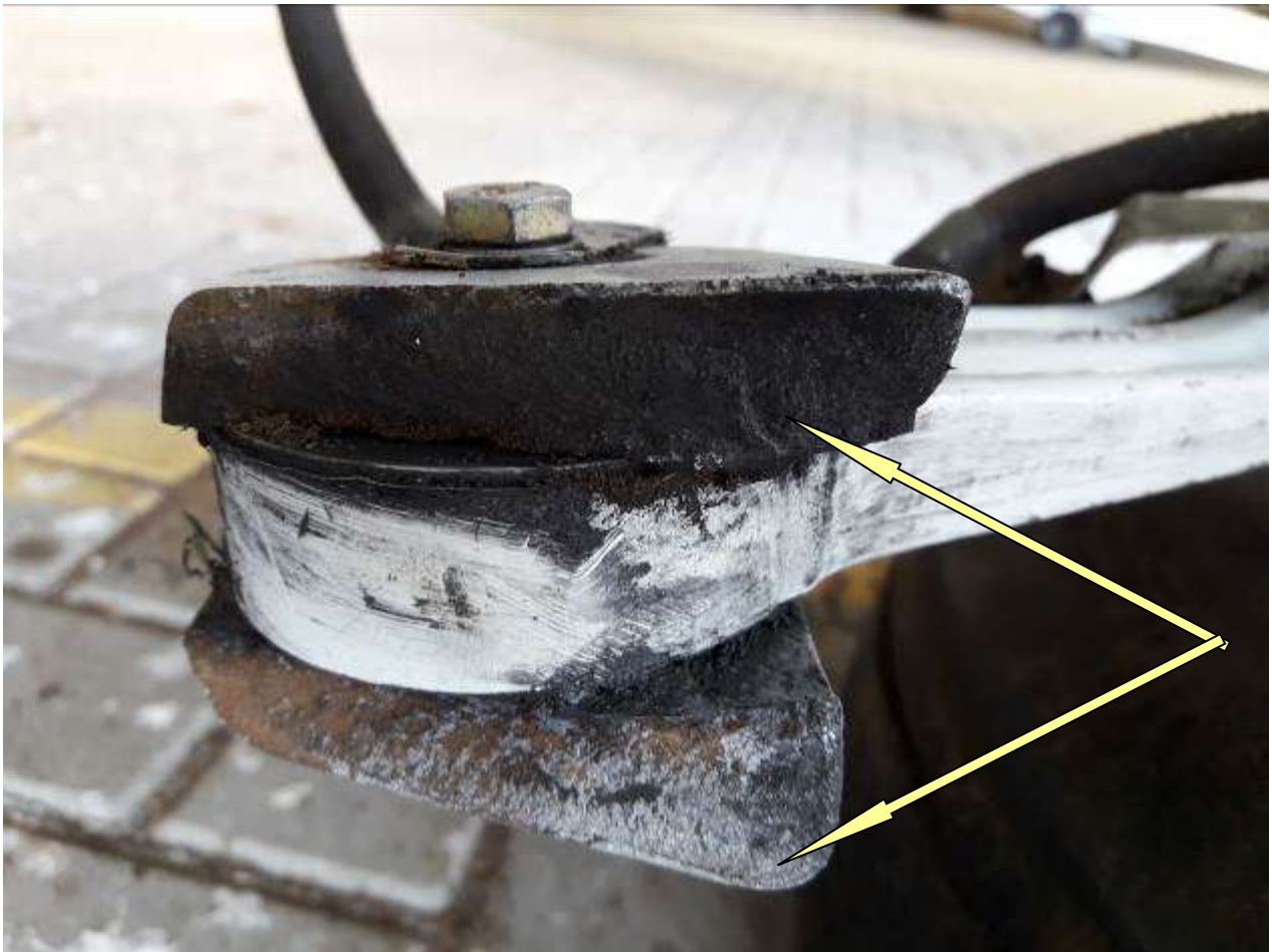
Figure 5. Broken-off torque link lugs (ear)
