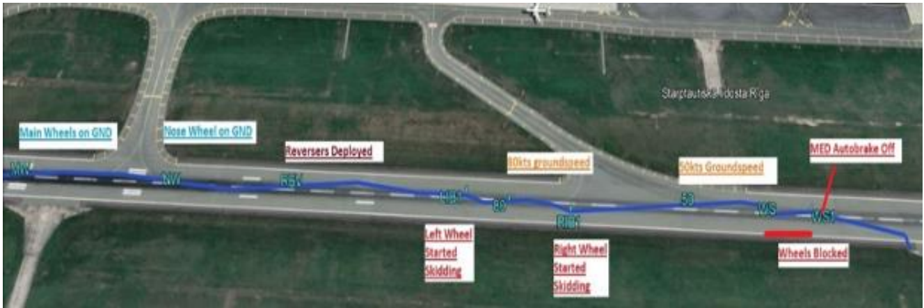
Figure 6: Computer simulated scheme of the aircraft deflection after landing on the RWY18
